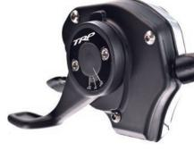
Shifter: Ergonomics are key to Aaron and he wanted something different for a reason. In addition to adjustability, TRP engineers looked at the cable release lever's ergonomics and devised a system to move it in a linear path to mimic the motion of a rider's thumb rather than rotating away.
